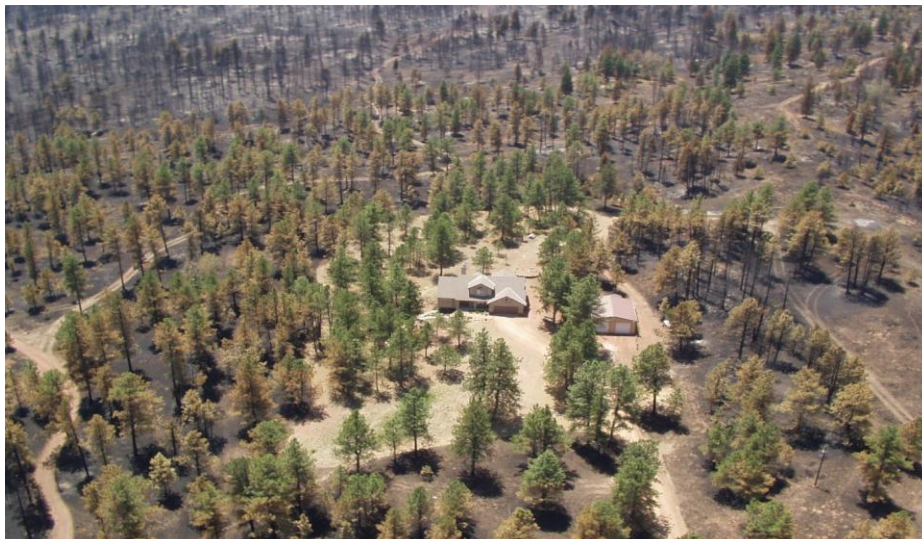
Figure 4: Survivable space around a home in the Hayman Fire. Note that zone one nearest the house did not burn. In zone two the fire burned on the ground but did not kill the trees. In the upper right a crown fire killed all the trees.
